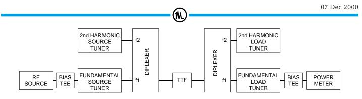
Figure 2: Passive Tuner System with 2nd Harmonic Source and Load Tuning
