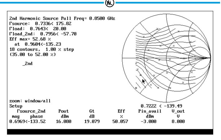
Figure 5: Efficiency vs. 2nd Harmonic Source Tuning
