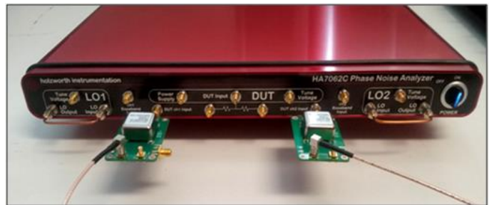
Figure 3: 100MHz OCXOs as DUT1 and DUT2
