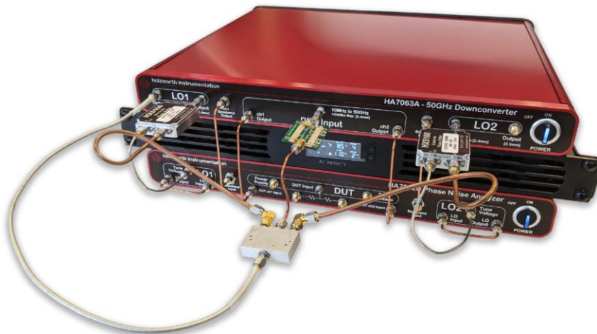
Figure 2: Residual measurement test setup of the HA7063A 50GHz Downconverter.
