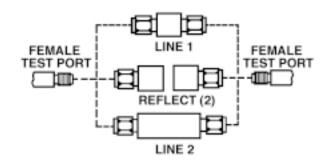
Figure 4(a): Basic LRL calibration procedure.
