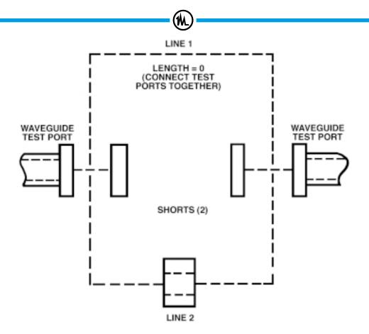
Figure 6: Basic LRL calibration in waveguide.
