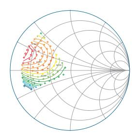
Example of noise parameters extracted from source pull measurements
