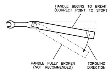
Figure 1. Using the Torque Wrench
