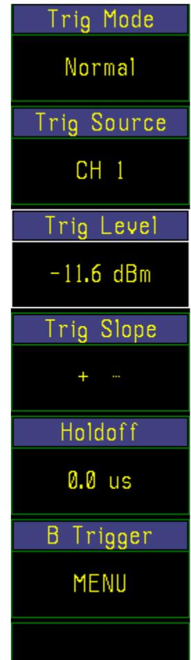
Fig 4-27c. Trig > menu Pulse; Normal trigger
