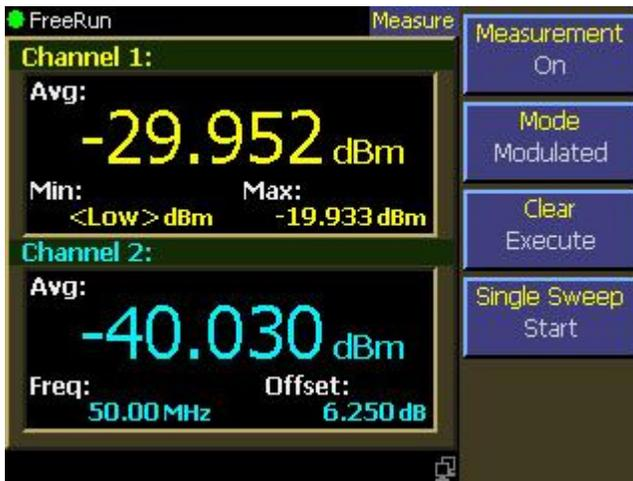
The measured result is the average power of the signal. Since the graphic display would basically just show a straight line, measurements in Modulated Mode use mainly the Numeric Display Mode.
