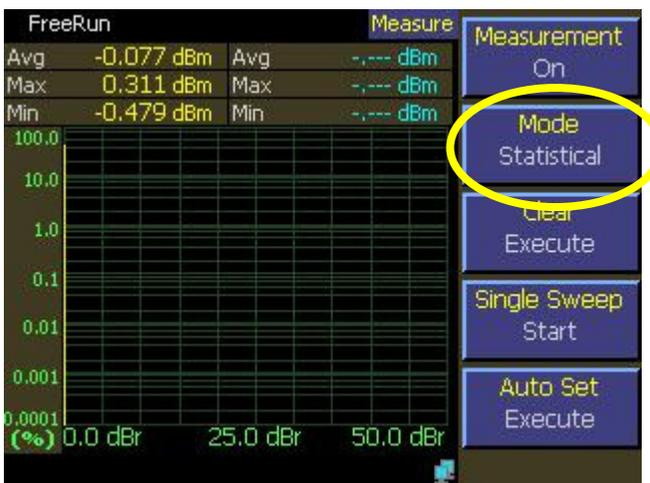
Statistical Mode is only available when a peak power sensor is connected to the 4540. It is the best choice for analyzing “noise-like” signals that are modulated in a random, non periodic fashion. Statistical mode yields information about the *probability of occurrence* of various power levels without regard for *when* those power levels occurred. Many digitally modulated spread-spectrum formats use a bandwidth coding techniques or many individual modulated carriers
