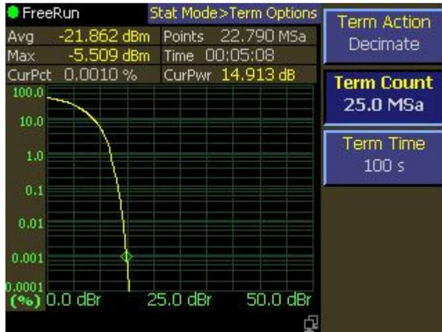
In a non-statistical peak power measurement the peak-to-average ratio is the parameter which describes the headroom required in linear amplifiers to prevent clipping or compressing the modulated carrier. The meaning of this ratio is easy to visualize in the case of simple modulation in which there is close correspondence between the modulating waveform and the carrier envelope. When this correspondence is not present, the peak-to-average ratio alone does not provide adequate information. It
