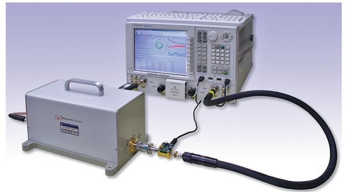
Figure 4. Photo of the new setup with the coaxial DUT.
