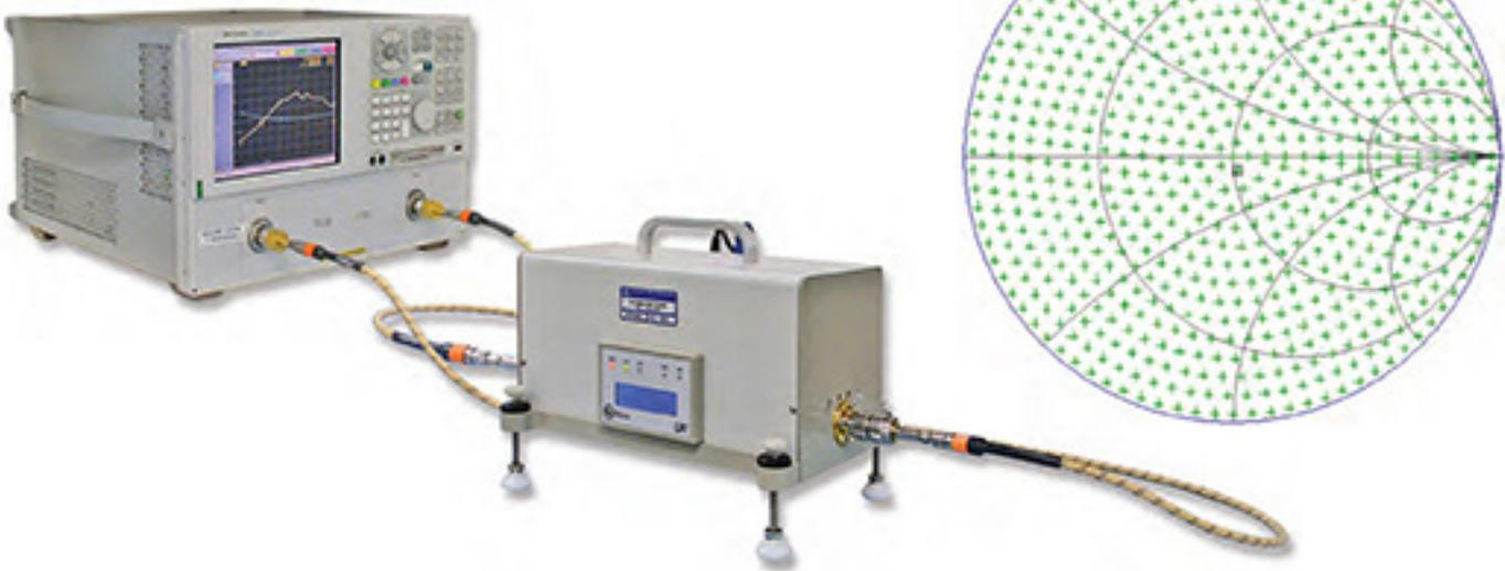
*Figure 3. An automated slide-screw impedance tuner setup with a calibrated VNA and automated software.*
