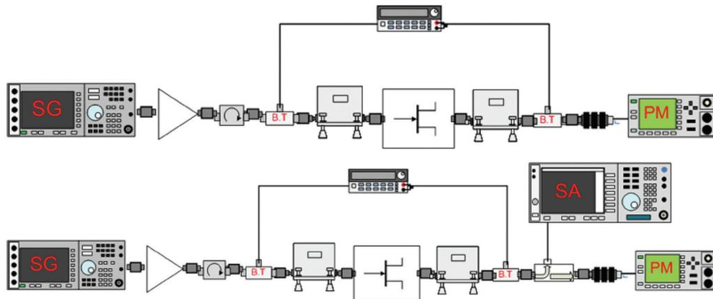
Figure 4. Traditional (scalar) load pull block diagrams.
