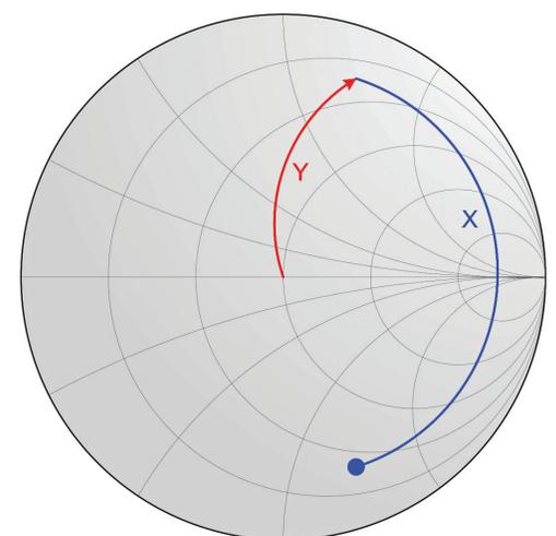
Figure 2. Effects of probe movement as shown on a Smith chart.
