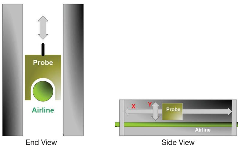
Figure 1. Simplified representation of a typical slide-screw tuner.
