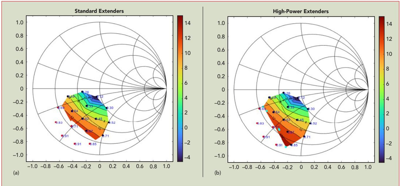
**▲ Fig. 7** (a) Load-pull iso-contours for output power using standard extender modules at 140 GHz. (b) Load-pull iso-contours for output power using -HP2 high-power extender modules at 140 GHz.
