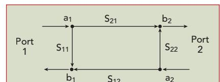
▲ Fig. 1 Two-port network representation of DUT.
