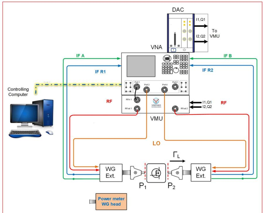
▲ Fig. 2 mmWave and sub-THz active load-pull system block diagram.
