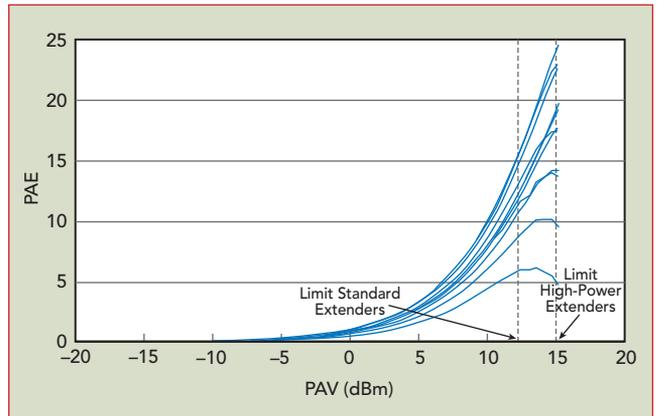
▲ **Fig. 6** PAE power sweep measurements at 140 GHz.
