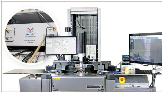
▲ Fig. 9 Active load-pull system with characterization software.
