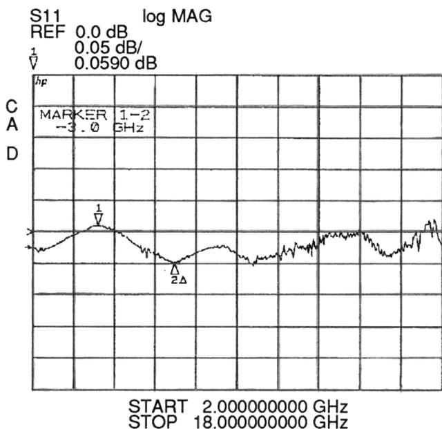
Figure 5. S11 (Log Magnitude) plot of a 2.498 cm Offset Short (7mm Connector)
