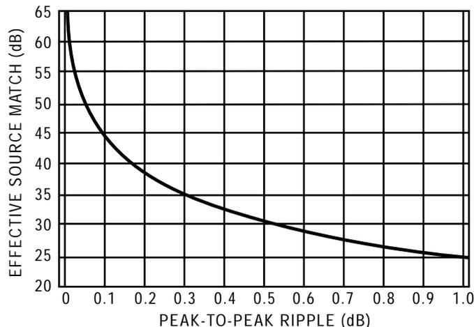
**Figure 3. Plot of Effective Source Match Versus Peak-to-Peak Trace Ripple**
