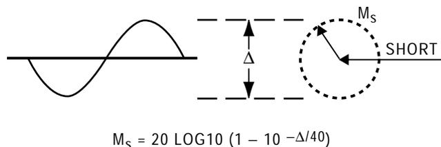
**Figure 2. Trace Ripple in a S11 Plot Due to Rotation of the Source Match Vector**
