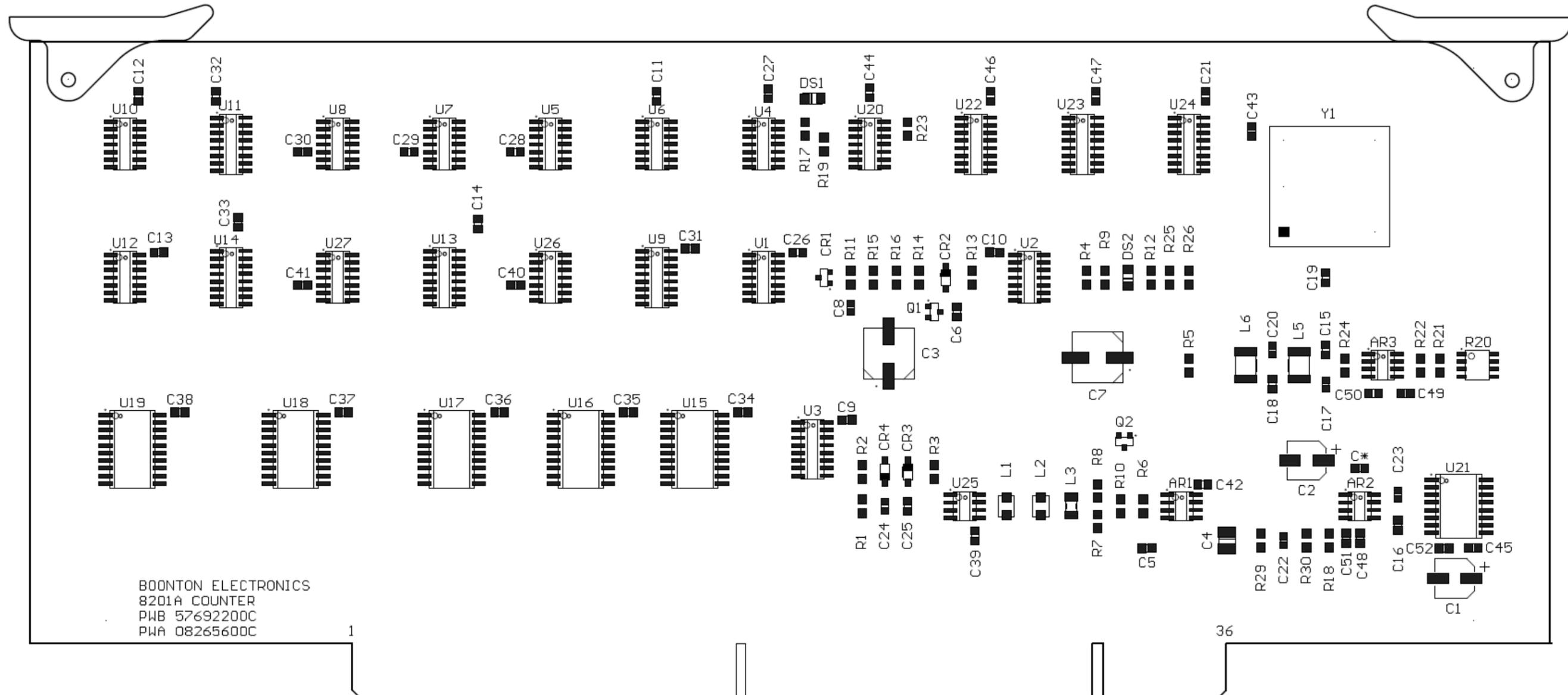
Figure 8-22 Counter Board A10, Parts Location
