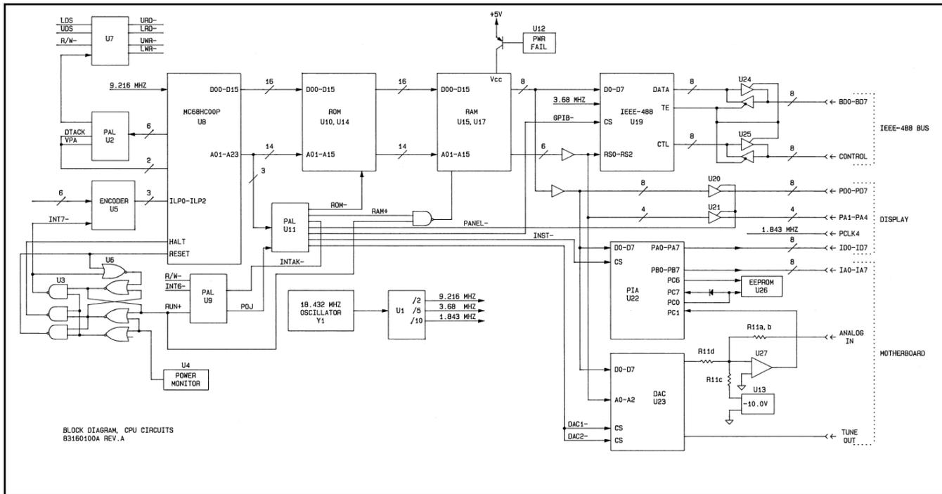
**FIGURE 4-10. CPU Circuits Block Diagram.**
