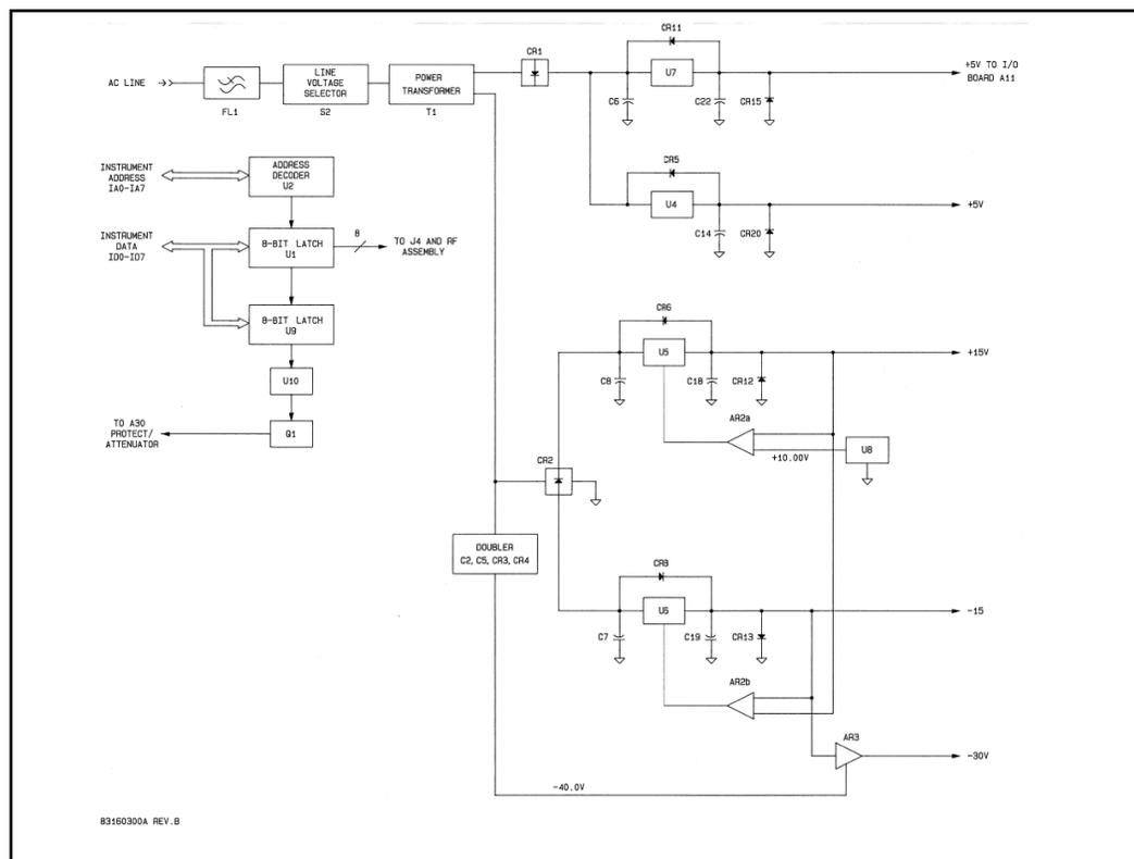
**FIGURE 4-13. Motherboard/Power Supply Block Diagram.**
