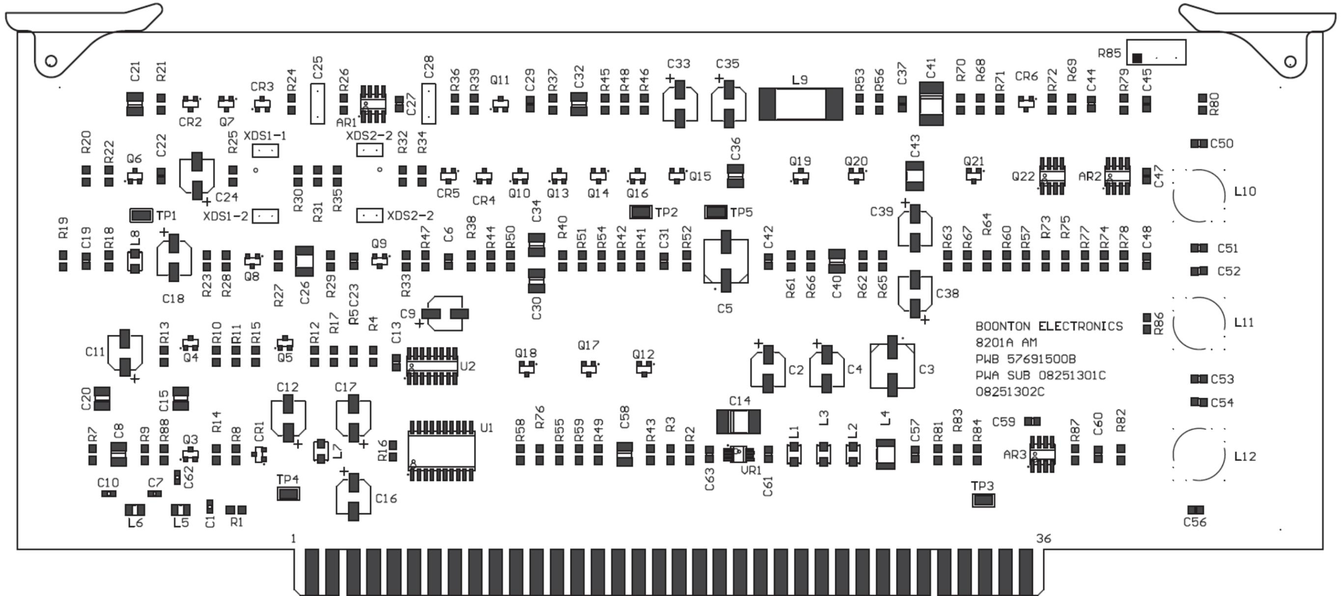
Figure 8-12. AM Board A5, Parts Location
