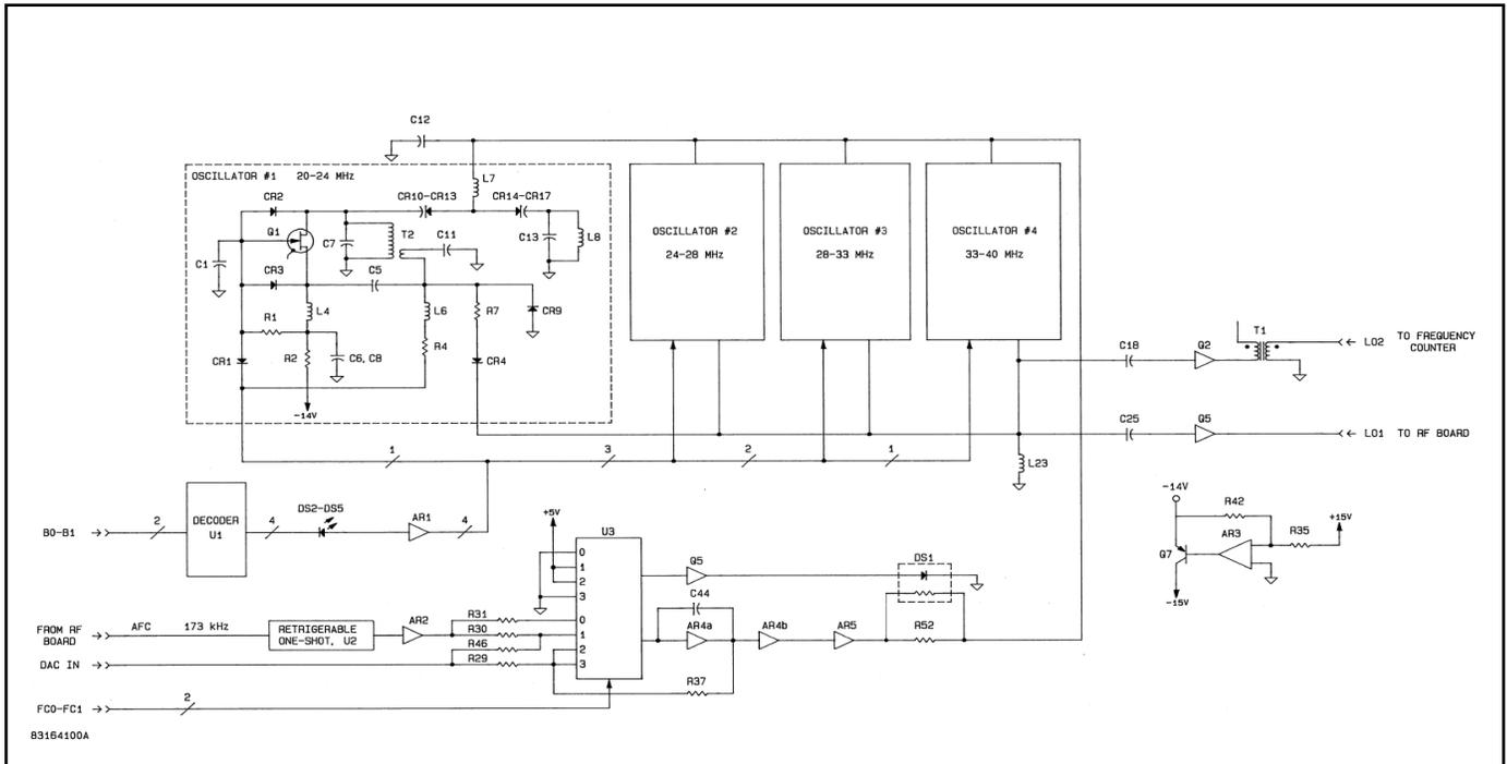
FIGURE 4-4. Local Oscillator Circuits Block Diagram.
