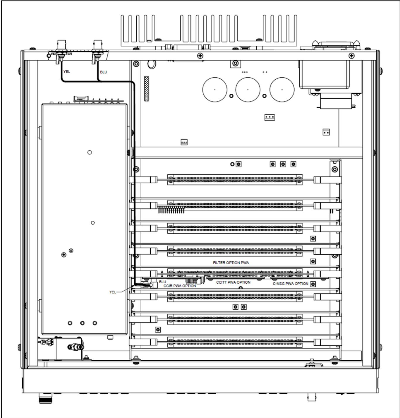
Figure 2-2. Optional Filter Installation
