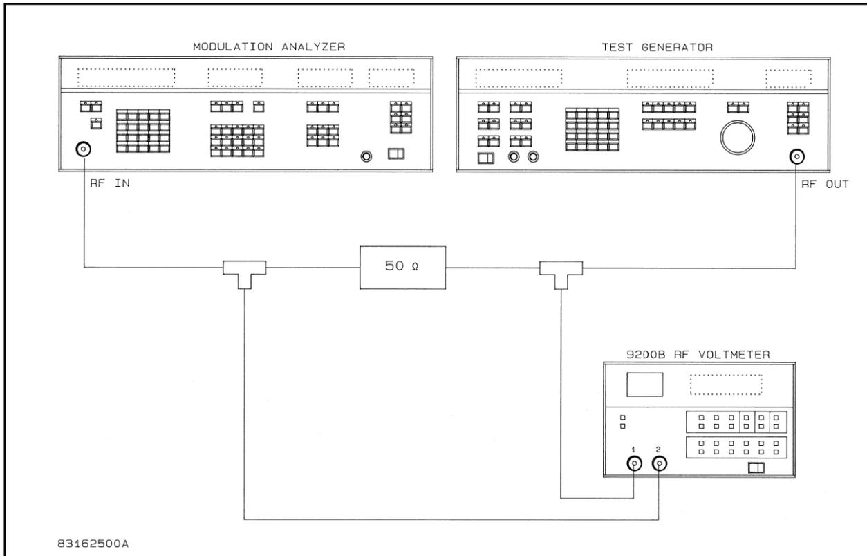
**FIGURE 5-3 Measurement Setup #3.**
