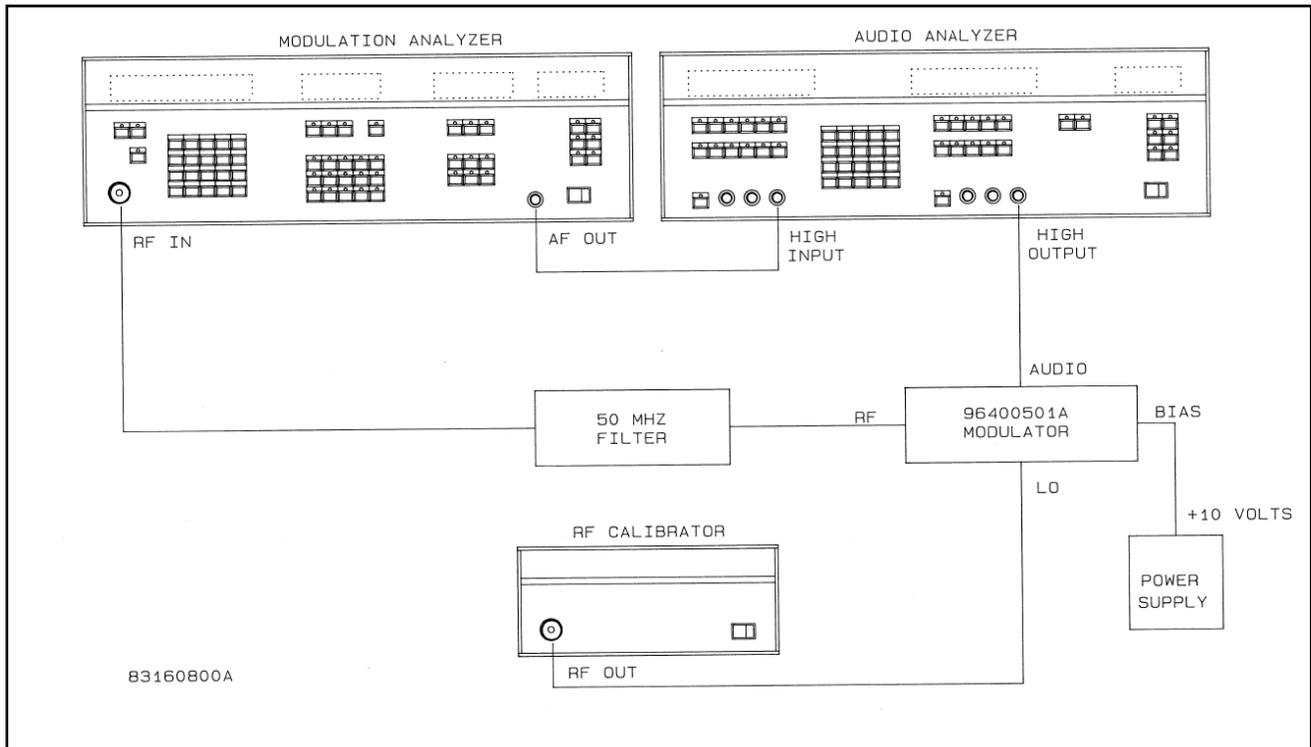
**FIGURE 5-1. Measurement Setup #1.**
