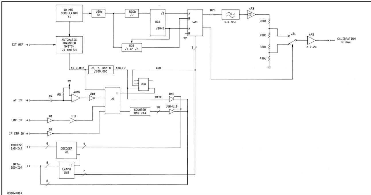
**FIGURE 4-11. Counter Circuits Block Diagram.**
