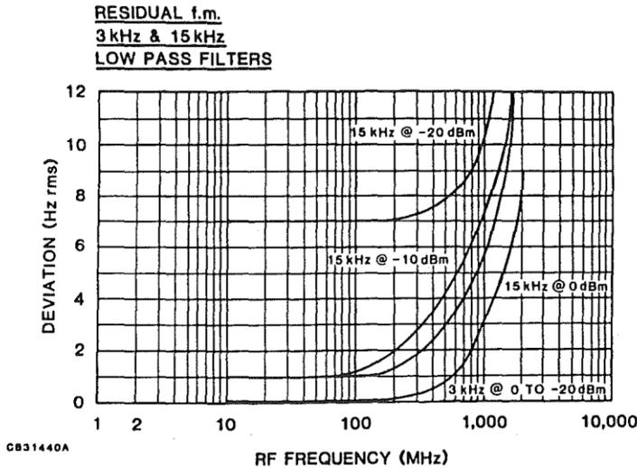
FIGURE 3-9. Residual FM, 3 and 15 kHz Filters.
