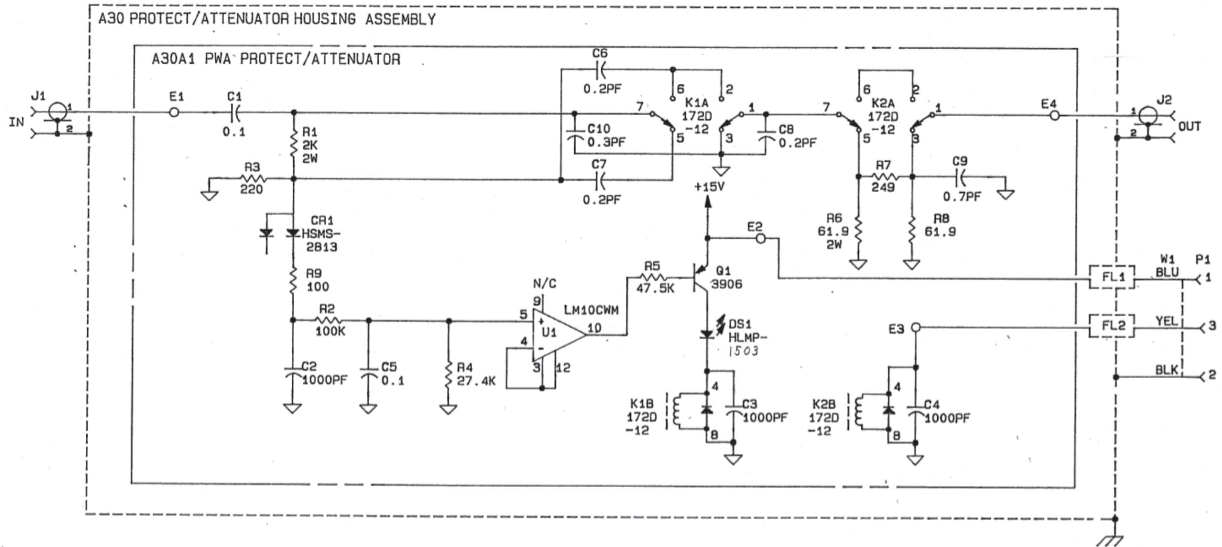
SCHEMATIC, 8201 PROTECT/ATTENUATOR PWB
