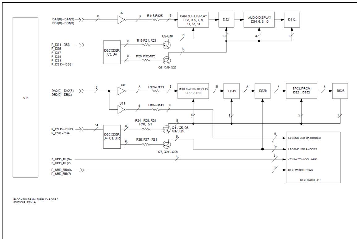
**FIGURE 4-12. Display and Keyboard Block Diagram.**
