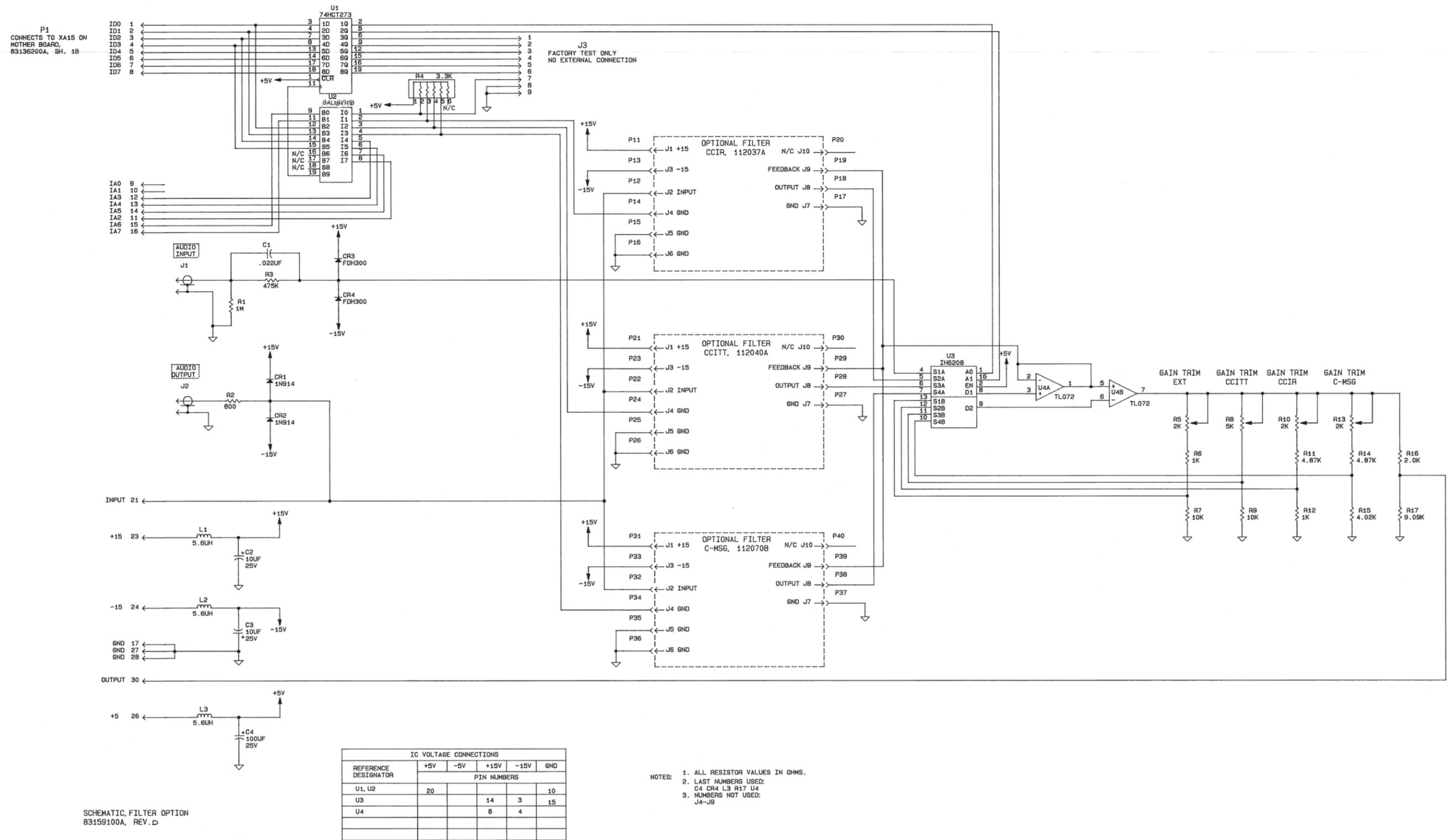
Figure 8-33. Option Board A15, Schematic Diagram
