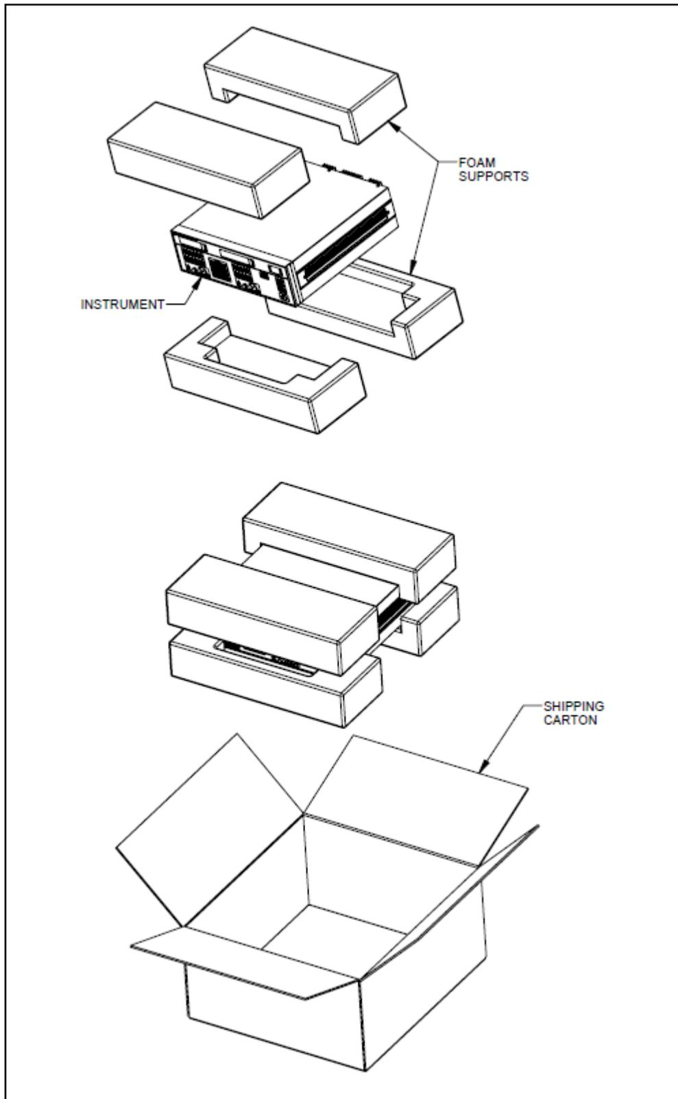
**Figure 2-1. Packing and Unpacking Diagram**
