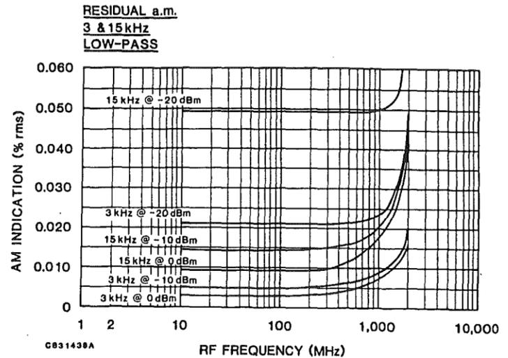
FIGURE 3-10. Residual AM, 3 and 15 kHz Filters.
