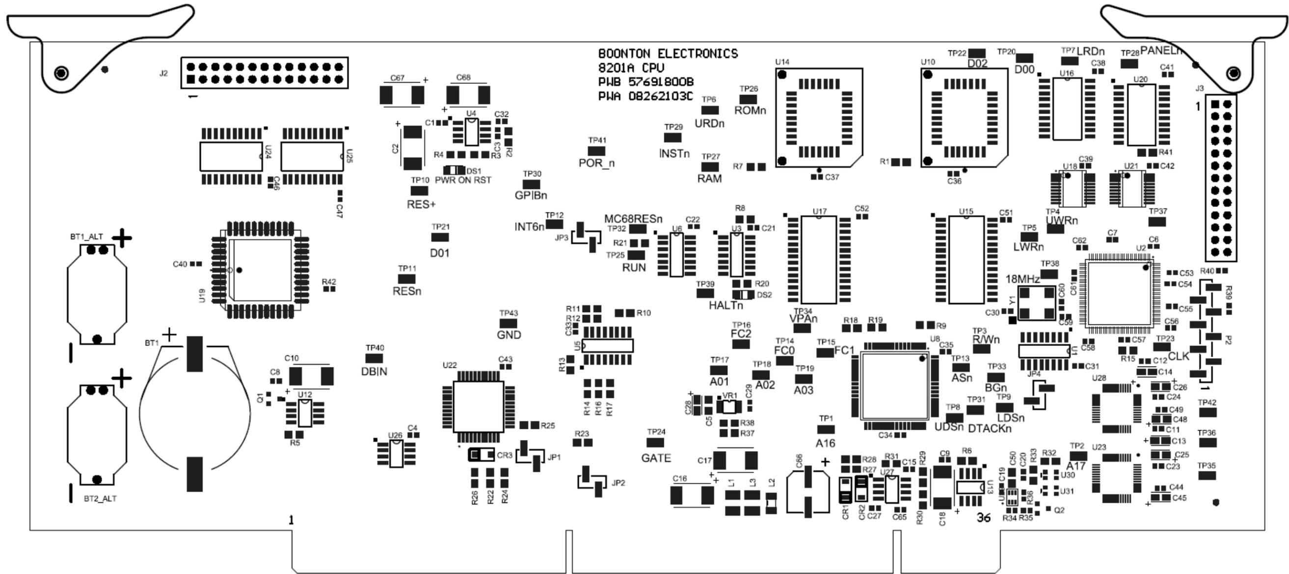
Figure 8-20. CPU Board A6, Parts Location
