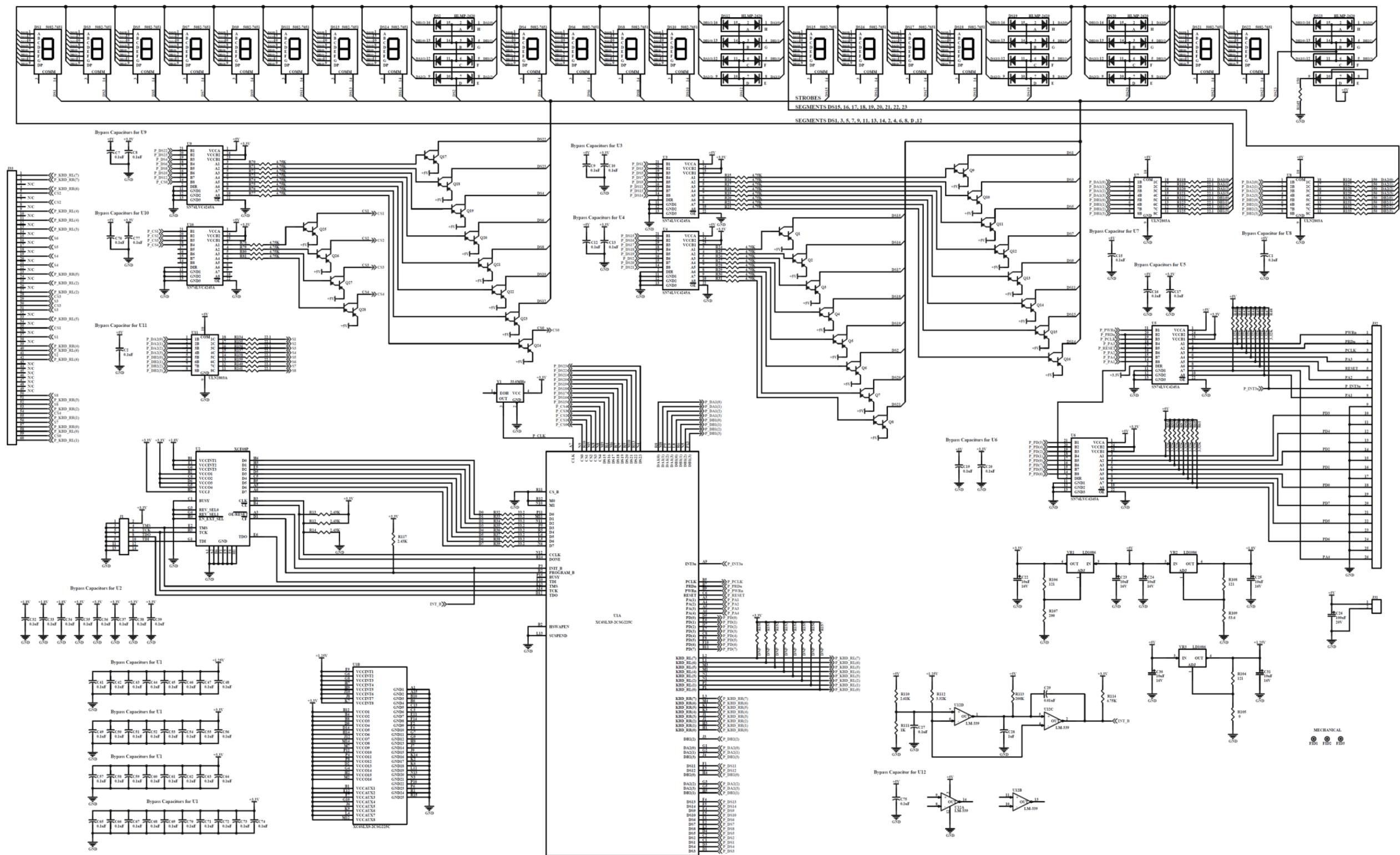
Figure 8-29. Display Board A12 Schematic
