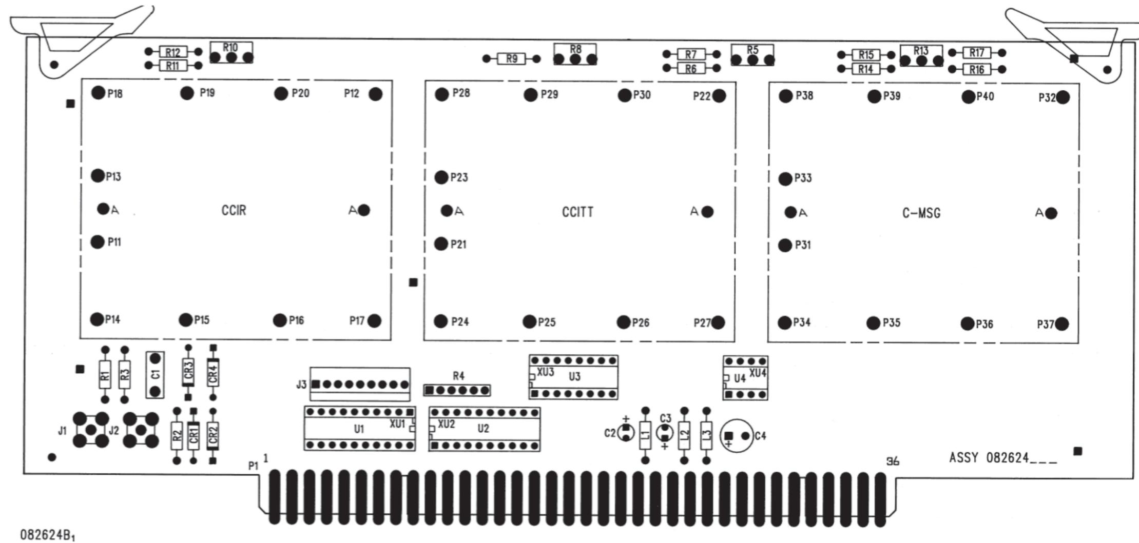
Figure 8-32. Filter Option Board A15, Parts Location
