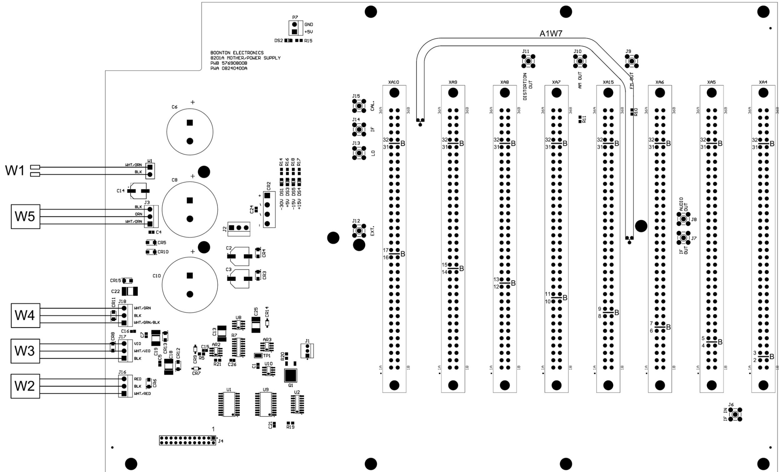
Figure 8-2. Mother/Power Supply Board A1, Parts Location.
