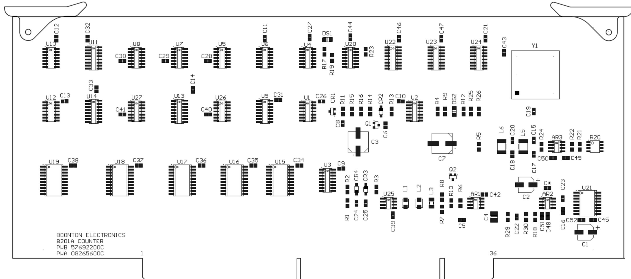
Figure 8-24 Counter Board A10, Parts Location
