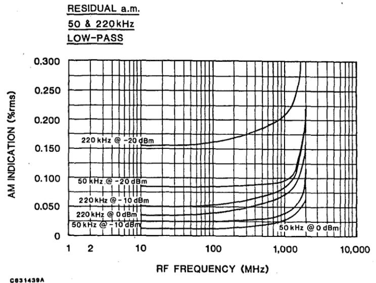
FIGURE 3-12. Residual AM, 50 and 220 kHz Filters.
