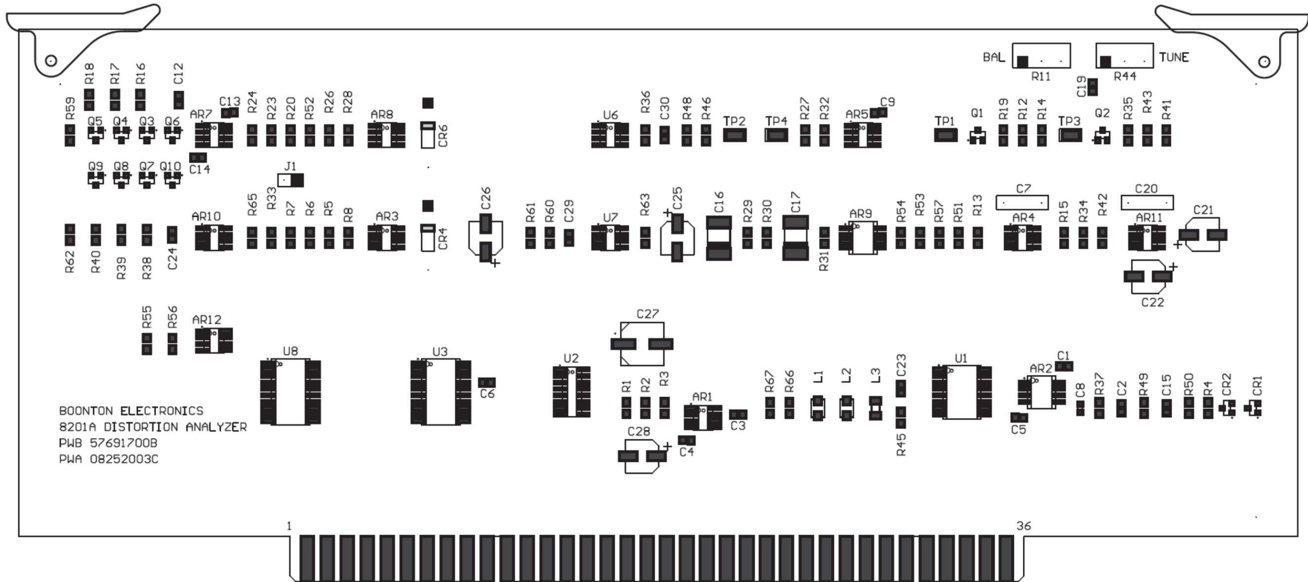
Figure 8-16. Distortion Analyzer A7, Parts Location
