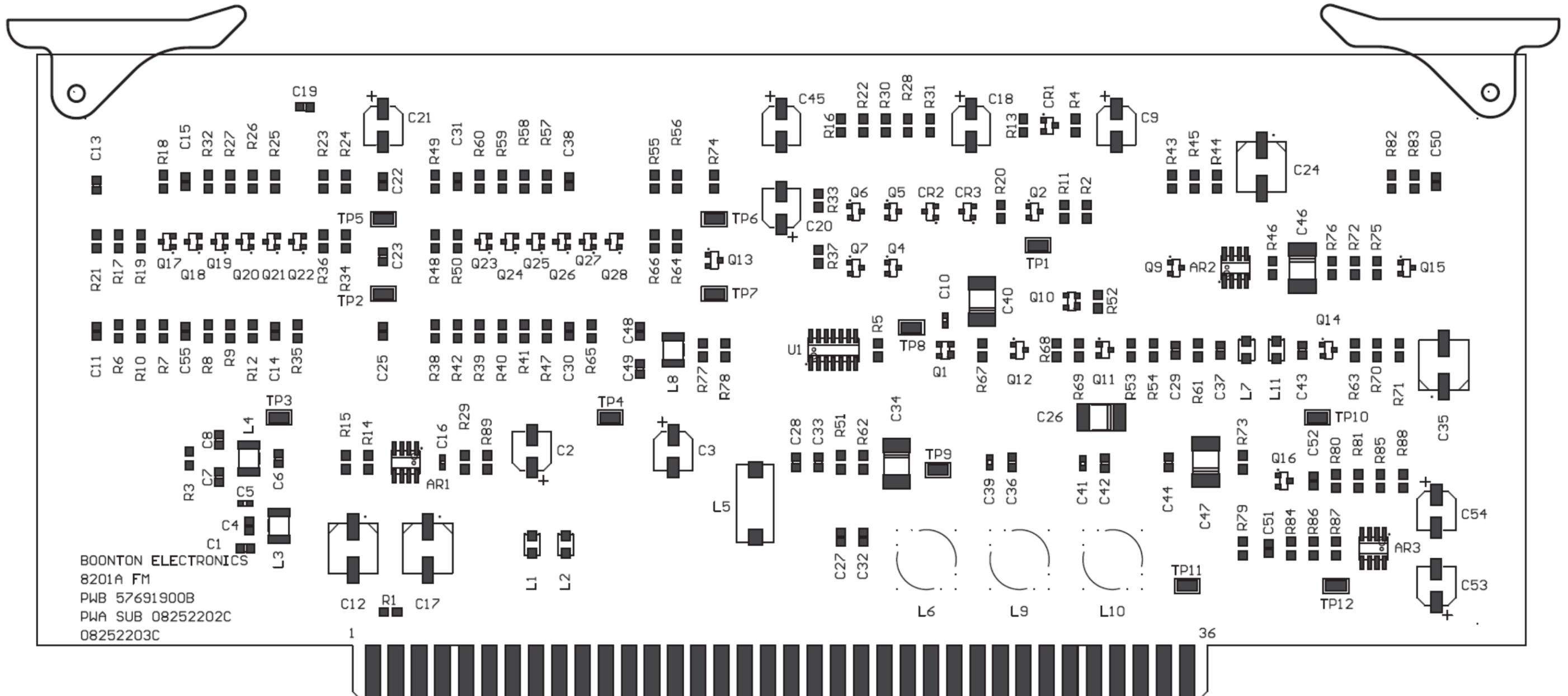
Figure 8-10. FM Board A4, Parts Location
