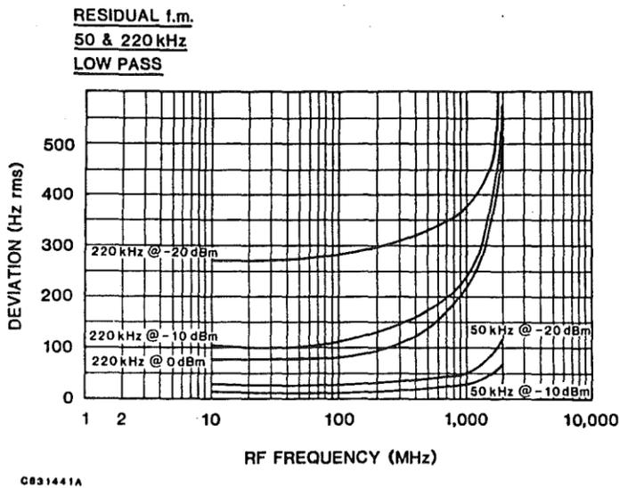
FIGURE 3-11. Residual FM, 50 and 220 kHz Filters.
