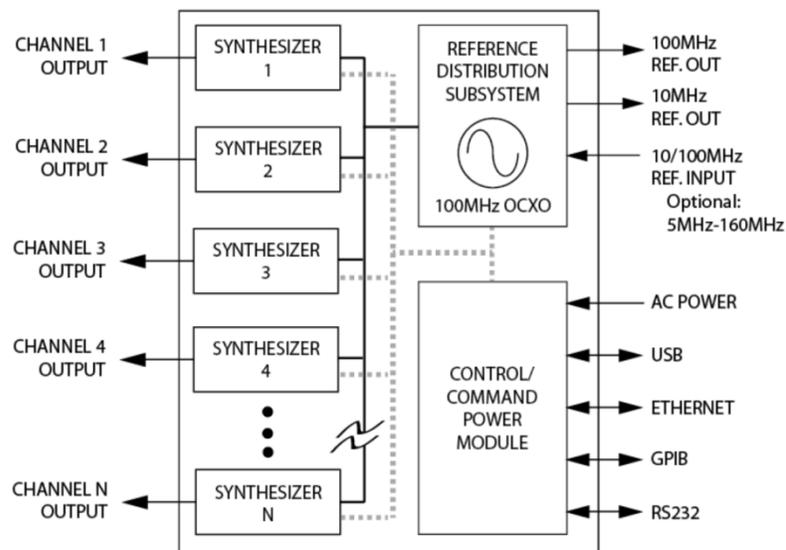
Holzworth Multi-channel RF Synthesizers offer the benefits of a proprietary NON-PLL based synthesis architecture. Coupling the NON-PLL architecture with a centralized reference distribution subsystem enables truly phase coherent, independently settable channels.
