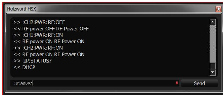
5. Begin by querying with the :IP:STATUS? command. Change status and/or re-configure the static network settings as necessary.
