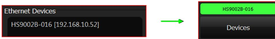
Identify the instrument by serial # or IP address and click to connect. If the connection is successful the window above 'Devices' will turn green (Ethernet) and display the instrument serial number:
