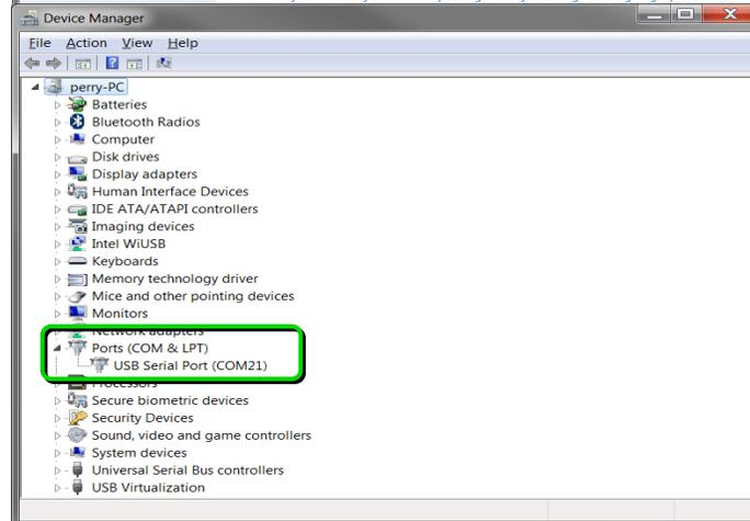
2. If the instrument is not present in Device Manager or in the Holzworth application GUI please unplug the USB cable and power cycle the synthesizer. Wait 5-10 seconds for the synthesizer to initialize an re-insert the USB cable. Click **Locate Devices**.
