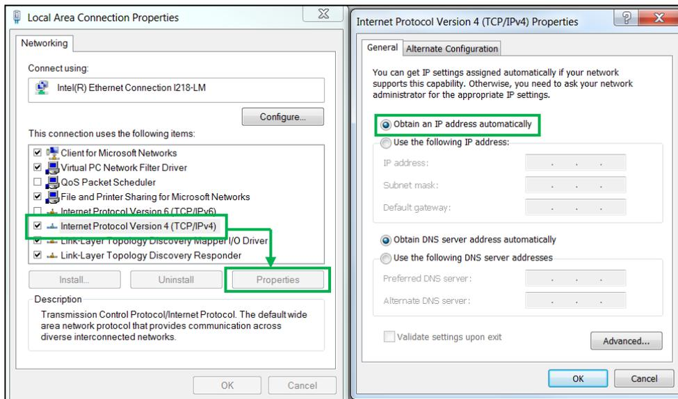
With a direct Ethernet connection between the PC and synthesizer both will default to network settings that will allow communication.
