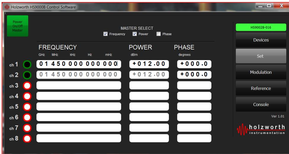
**NOTE** that the GUI does not specifically identify each channel frequency range, but the frequency limits of each loaded channel is auto-detected and hard set for each channel.
