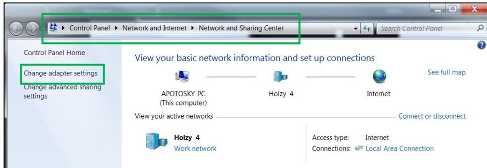
3. In the Change Adapter Settings window right click on any network connections that are not required for communication with the HA7062 and select Disable.
