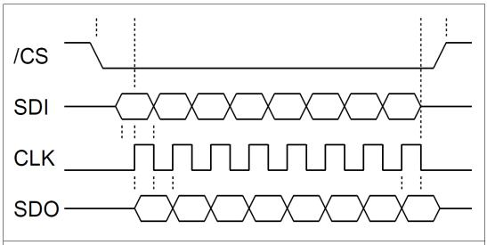
Bit level timing demonstrating where data is sampled into and out of the module on the rising edge of sclk. Data out is valid on the falling edge of sclk.
