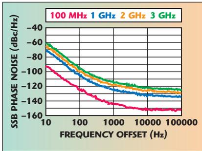
▲ Fig. 1 SSB phase noise at 100 MHz, 1 GHz, 2 GHz and 3 GHz ( $P_{out} = +12$  dBm).
