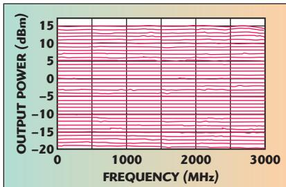
▲ Fig. 2 Output power flatness vs. frequency.
