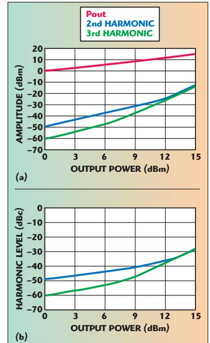
▲ Fig. 4 Absolute (a) and relative (b) harmonic data ( $F_0 = 1$  GHz).
