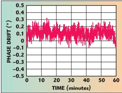
▲ Fig. 5 Channel to channel phase drift performance (3 GHz,  $20 \pm 2^\circ\text{C}$ )
