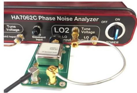
**Figure 2** The external LO mode function was developed primarily for evaluating crystal
