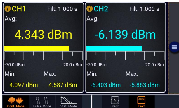
Figure 3-5. PMX40 Text Display Mode Using Continuous Measure Mode
