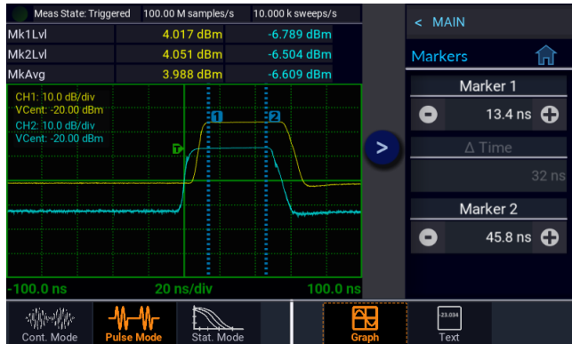
Figure 3-6. Marker Measurements on CH1 and CH2 Pulses
