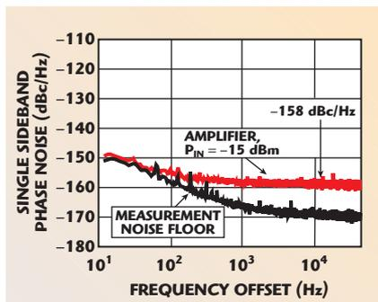
▲ Fig. 2 Measured additive phase noise of an amplifier with  $P_{in} = -15$  dBm.
