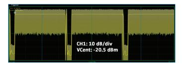
\* "Video bandwidth tested by measuring peak-to-average on a two-tone separation signal at +10dBm, frequency set at 1 GHz. Test limit set at 2 dB roll off from the nominal 3dB peak-to-average flatness graph"
