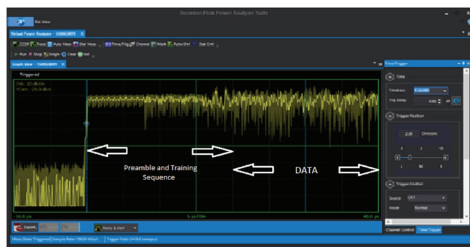
Figure 3. A typical Wi-Fi 802.11ac signal measured by the Boonton 55006 Peak Power Sensor:
