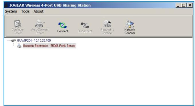
Figure 4. Status of a WiFi-USB hub before Boonton USB sensor is selected and connected
