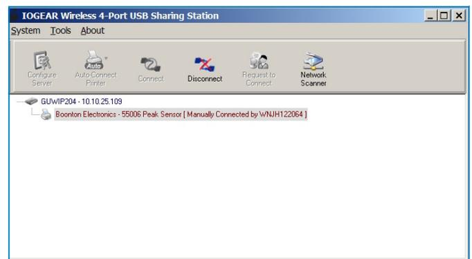
Figure 5. Status of the utility software once USB sensor remote connection is established
