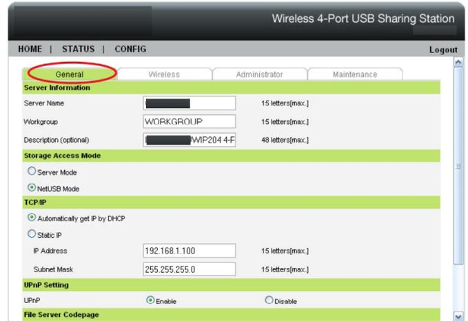
Figure 2. IP address (DHCP or Static) configuration by using an Ethernet connection to the USB sharing hub
