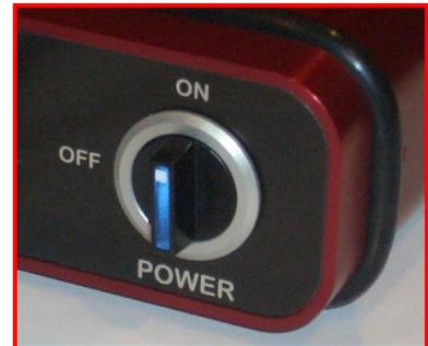
The master power switch located at the right side of the front panel is equipped with a blue indicator light which illuminates when the DC power is active.
