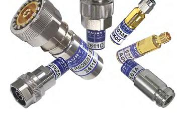
Precision standard mismatches are fixed coaxial terminations, which are used to introduce a known VSWR into a 50 ohm transmission system. These mismatches are extremely useful in a wide variety of applications and are quick and easy to use. They can be used to calibrate swept reflectometers, verify network analyzer calibration, establish impedance references in TDR measurements, etc.
