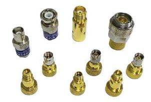
Shielded, coaxial opens are used in the calibration of vector network analyzers to provide a nominal 180° phase offset from a compatible reference short over a wide range of frequencies.
