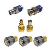
Fixed flush and fixed offset short circuit terminations (shorts) are used to establish reference planes in transmission systems and as key elements in the calibration of vector network analyzers (VNAs). Offset shorts can be used for banded calibrations of VNA. Those with the longest offset are often used to evaluate the calibration effectiveness of a VNA by measuring the effective source match after calibration.
