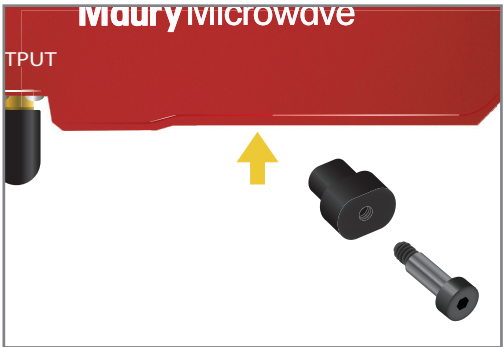
Lock screw/plug storage location (Underneath Tuner)
