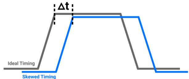
Combining this performance with the fastest measurement rate of 100,000 per second, 100 picosecond time resolution, and superior trigger stability, the RTP5000 Series can also measure any delay experienced at various points along a satellite communications path. Clients can even use their actual signals during testing to pinpoint delay and apply the necessary corrections.
