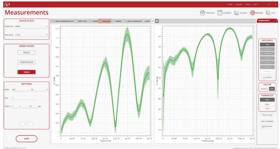
Figure 7. Example measurement uncertainty plot using Insight.
