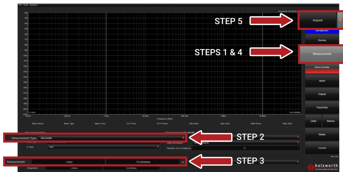
Figure 8: Configure the measurement type, frequency span, and display area before acquiring an absolute phase noise measurement.
