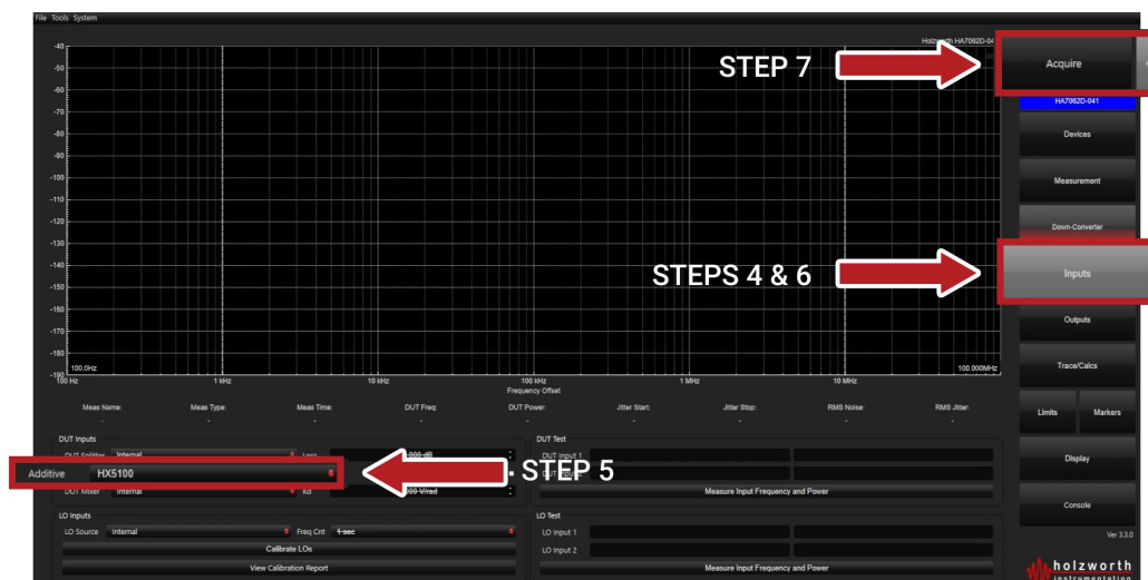
Figure 12: Configuring the Inputs menu and acquiring the additive phase noise measurement.
