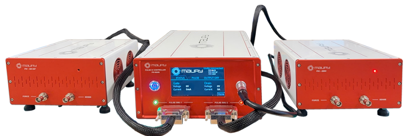
Figure 2. Maury PIV Series pulsed IV measurement system.
